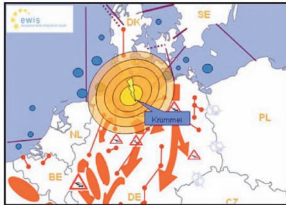
Voltage dip during a three phase short circuit in the German grid
